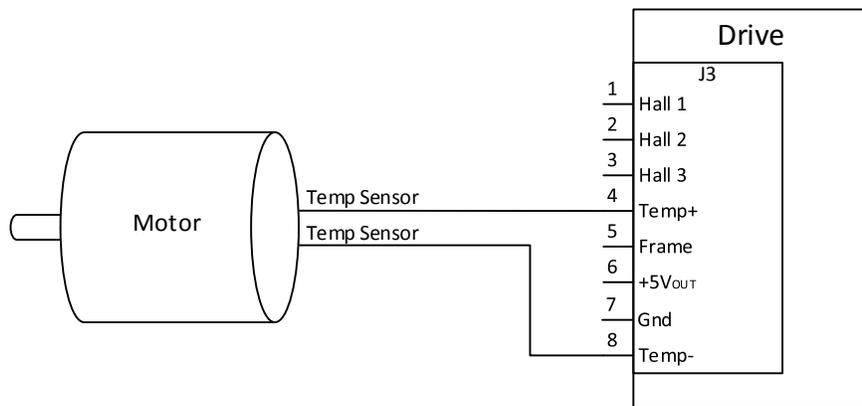
Figure 17: Temperature sensor connection to the drive
