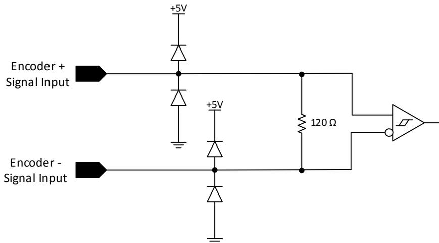
Figure 16: Encoder signal-ended input circuit
