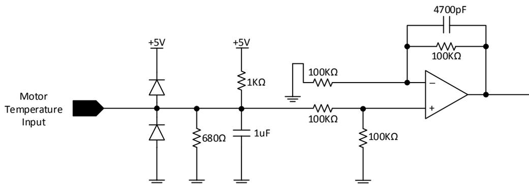
Figure 18: Temperature sensor signal input circuit
