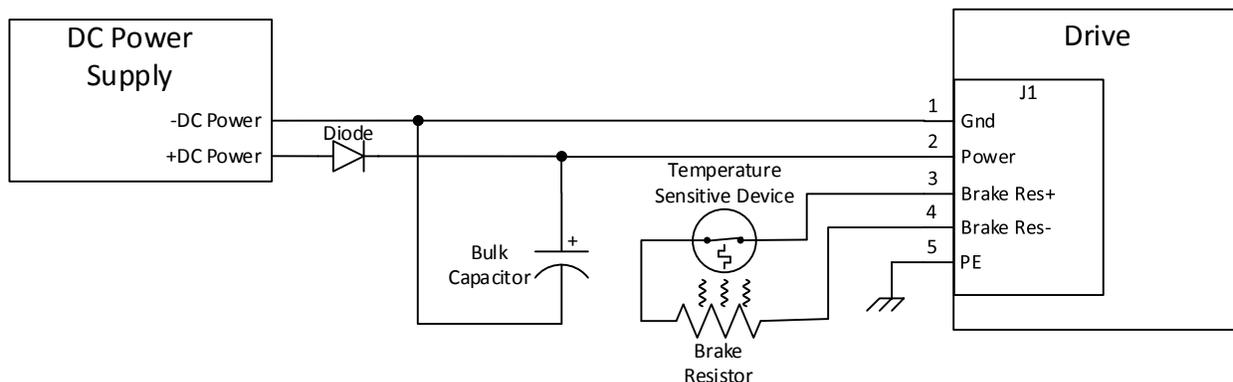
**Figure 26: External brake resistor and bulk capacitor connection to the drive**
