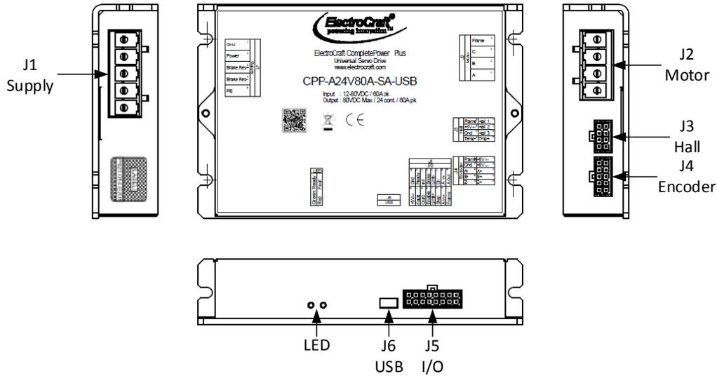
Figure 9: Drive connector layout
