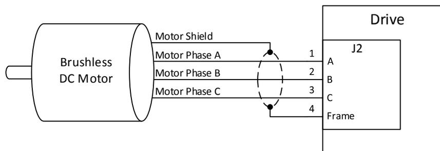
Figure 11: Brushless DC motor connection to the drive
