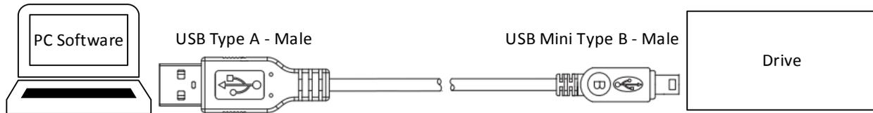
Figure 24: USB cable connection between computer and drive
