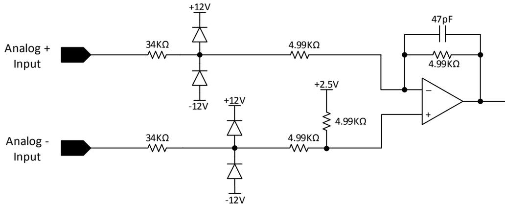
**Figure 22: Analog input circuit**
