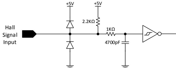
Figure 13: Hall sensor signal input circuit
