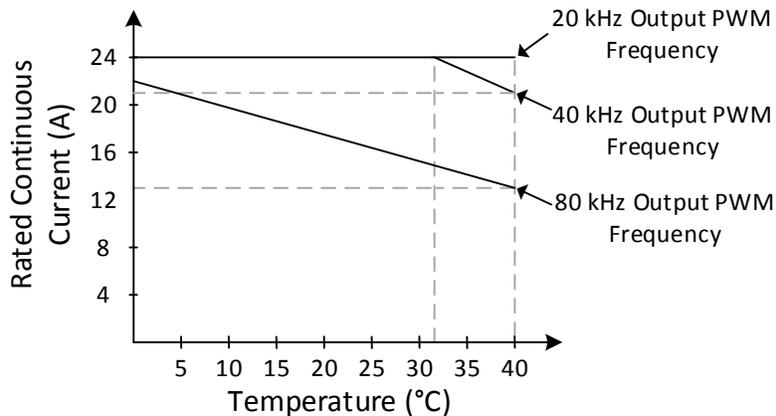
Figure 6: Drive temperature derating at 80VDC
