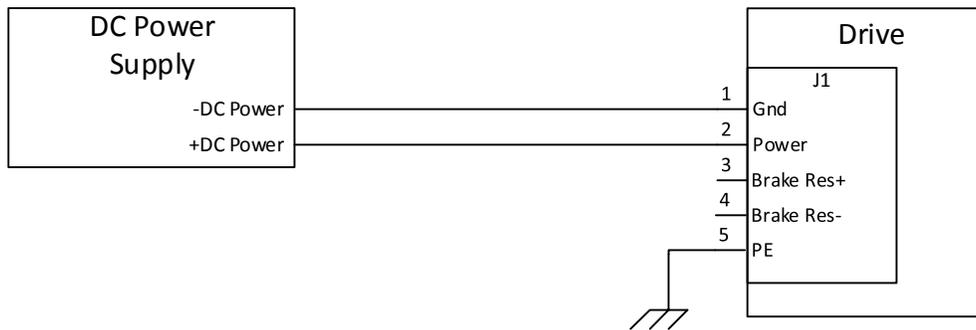
Figure 10: Power supply connection to the drive
