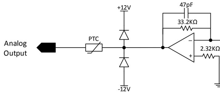
**Figure 23: Analog output circuit**
