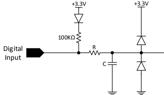
Note: For Step and Direction digital inputs  $R = 10K\Omega$  and  $C = 10pF$ . For In 0, Enable, Brake, Limit Switch Positive and Limit Switch Negative digital inputs  $R = 20K\Omega$  and  $C = 4700pF$ .
