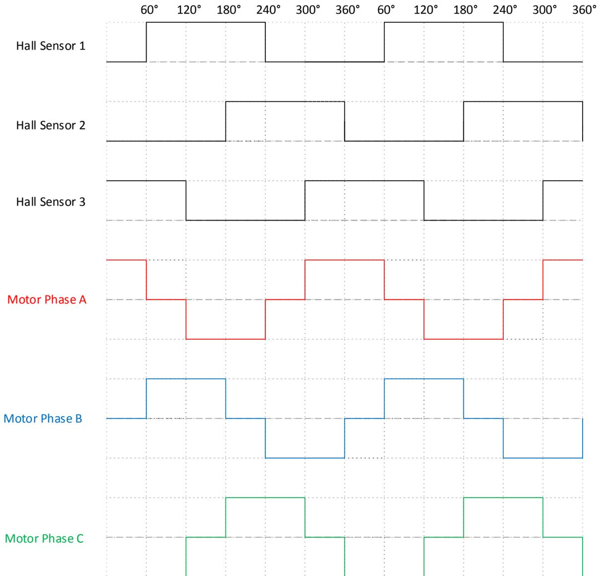
Figure 2: Trapezoidal Commutation with Hall sensor feedback
