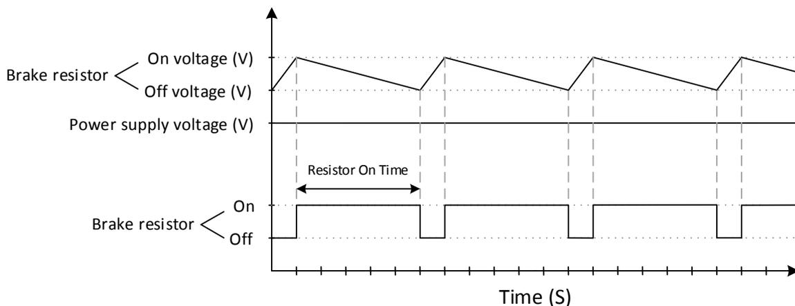
**Figure 25: Brake resistor operation graph**
