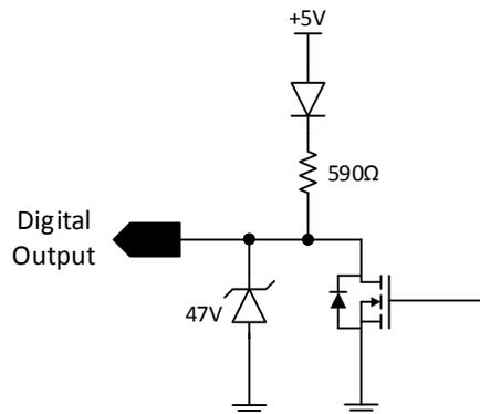
Figure 21: Digital output circuit
